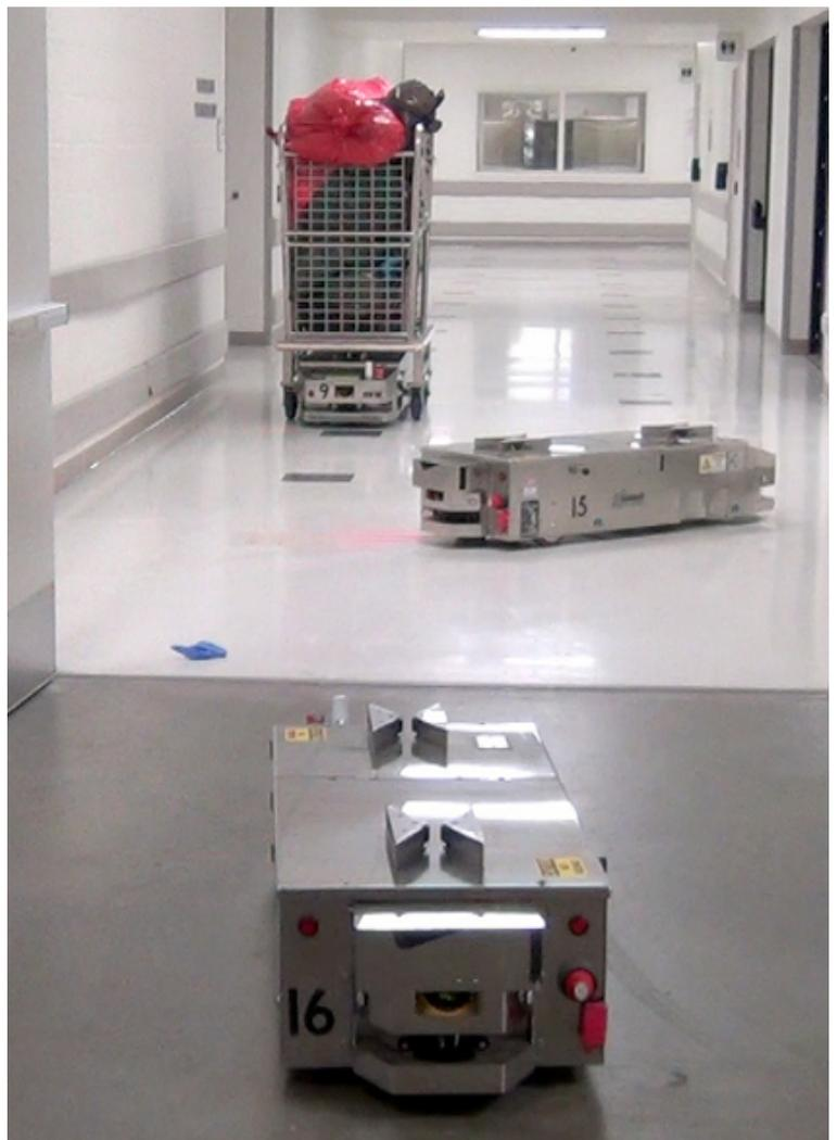
**M**anual cart transportation is not only wasteful and inefficient but also completely avoidable today thanks to mobile robots. These battery-powered machines, commonly referred to as automatic guided vehicles (AGVs), are capable of performing a wide variety of tasks within healthcare facilities.
